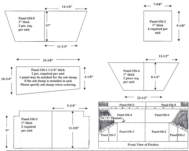
There are 12 refractory panels. The refractory panels can be installed either side out.
