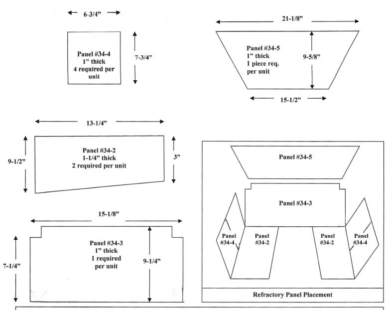
There are a total of 8 refractory panels. The refractory panels can be installed either side out.
